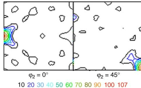
Fig. 3. ODF of sample strained in RD,  $\epsilon = 0.23$ .
