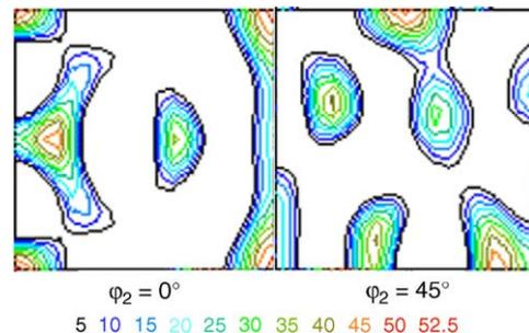
Fig. 5. ODF of strained sample ( $\epsilon = 0.23$  on TD).
