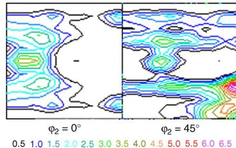
Fig. 4. ODF of annealed sample ( $\epsilon = 0.23$  on RD).
