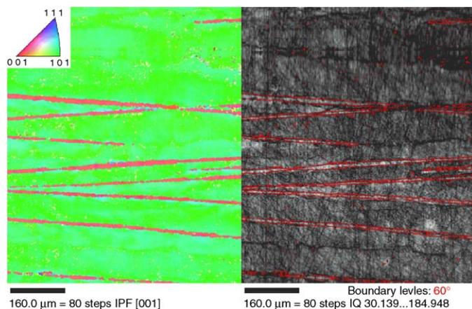
Fig. 7. Deformation twins in the sample strained to 23% in the rolling direction (RD).
