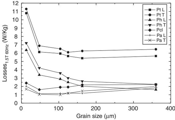
Fig. 1. Effect of grain size in the different losses components  $P_t$ ,  $P_h$ ,  $P_a$ , and  $P_{cl}$ , in the transverse (T) and longitudinal (L) directions.
