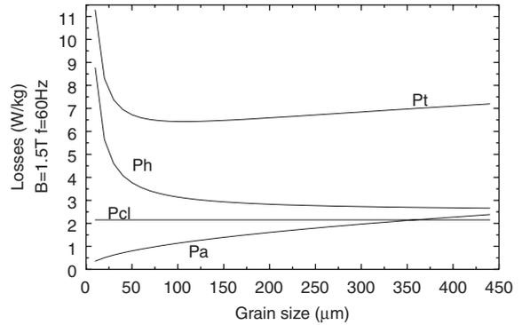
Fig. 4. Result of application of the model described in Section 3.3. Effect of the grain size the different losses components  $P_t$ ,  $P_h$ ,  $P_a$ , and  $P_{cl}$ . Transverse direction.
