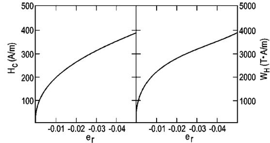
FIG. 4. Computed plots of  $H_c$  vs  $e_r$  and  $W_H$  vs  $e_r$ . In this plot, it is seen that a Ludwik exponent  $n=\frac{1}{2}$  results in both  $H_c$  and  $W_H$  having an  $e_r^{1/2}$  dependence.
