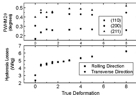
FIG. 1. Hysteresis loss  $W_H$  vs  $e_r$  and FWHM of x-ray peaks for different crystalline planes plotted against residual strain  $e_r$ . X-ray diffraction data obtained under Cu  $K_\alpha$  radiation, 40 kV, 20 mA.
