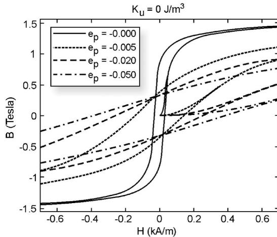
FIG. 3. Computed hysteresis curves using Ludwik's equation for  $\sigma_F$  vs  $e_r$  with  $n=1/2$  and using the new expression for residual stress  $\sigma_r$ . Hysteresis curves are shown for zero deformation and for deformations of 0.005, 0.02, and 0.05. The loops at nonzero deformations are not shown in full, as they are cut off at  $H_{max}=700$  A/m.
