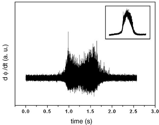
Fig. 1. Barkhausen noise signal for non-oriented electrical steel obtained at 200 mHz. Inset: original curve before the subtraction of the base line.
