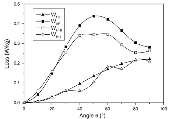
Fig. 2. Angular behaviour of the anisotropic part of the inclusion ( $W_{f_\theta}$ ) and texture ( $W_{E_A}$ ) component of the total losses, as determined by the inclusion/texture model, compared to the high-induction ( $W_{HHI}$ ) and low-induction ( $W_{HLI}$ ) components of the hysteresis loss, as determined by the graphical separation of hysteresis loss.
