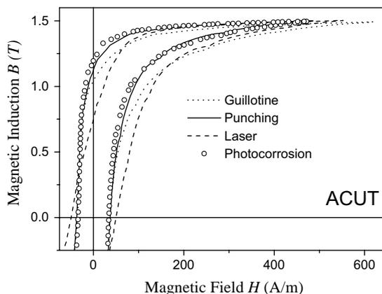
Fig. 3. Quasi-static hysteresis curves of samples cut by different techniques, in the annealed + cut condition.
