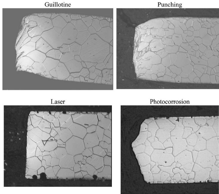
Fig. 1. Edge profiles before annealing.
