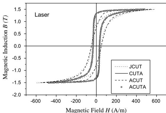
Fig. 2. JCUT, CUT+A, A+CUT, A+CUT+A quasi-static hysteresis curves of samples cut by laser.
