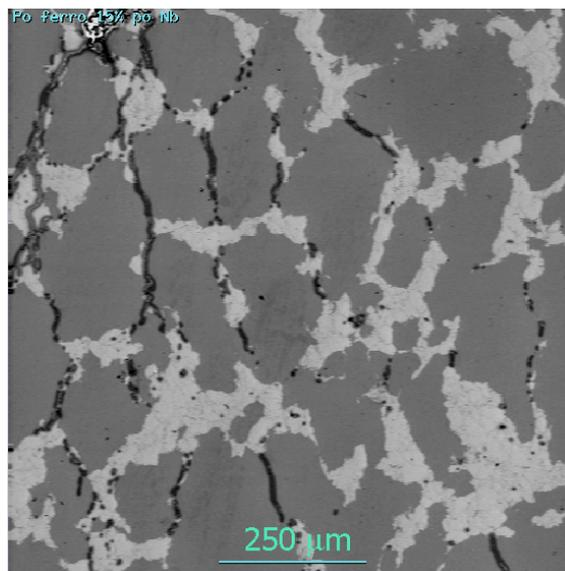
Figure 1. Microstructure of sample 15T. Secondary electrons image in SEM. White areas are Nb (+N). Fe particles are predominantly isolated.
