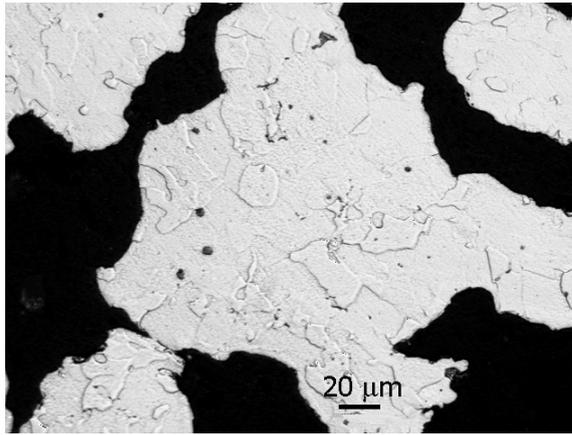
Figure 2: Iron particles etched with nital.
