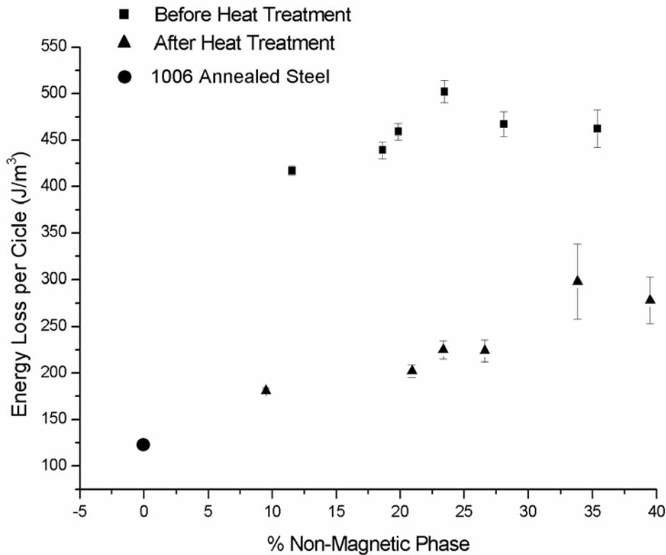
Figure 7. Effect of non-magnetic phase volume fraction energy loss per cycle at 0.5T
