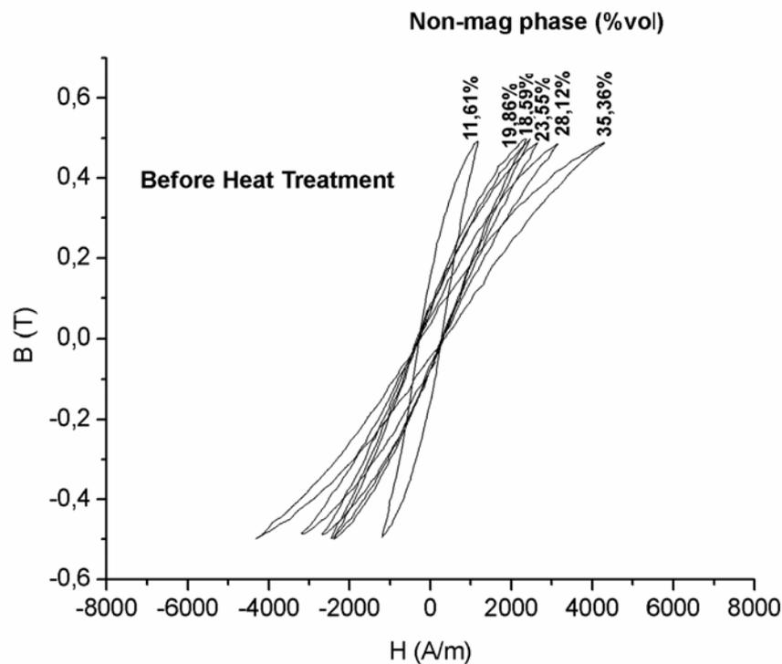
Figure 4. Quasi-static hysteresis curves for as-pressed samples
