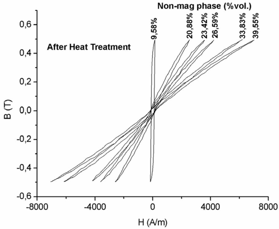
Figure 5. Quasi-static hysteresis curves for annealed samples
