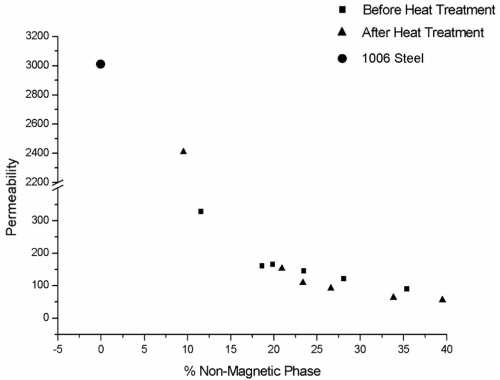
Figure 6. Effect of non-magnetic phase volume fraction on on magnetic permeability at 0.5T
