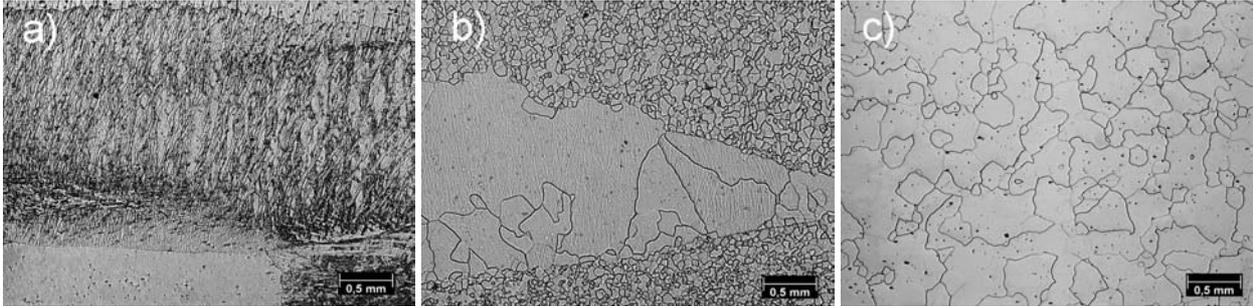
Fig. 1. Optical micrographs of the microstructure after first cold rolling (a), intermediate annealing (b), and final annealing (c)
