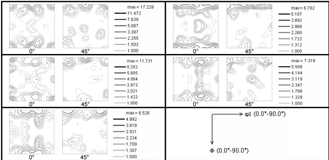
Fig. 4. ODF of final annealed sample measured by EBSD,  $\phi_2$  ( $0^\circ$  and  $45^\circ$ ) sections.
