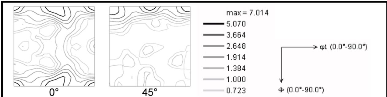
Fig. 5. Average ODF of final annealed sample measured by EBSD,  $\phi_2$  ( $0^\circ$  and  $45^\circ$ ) sections.
