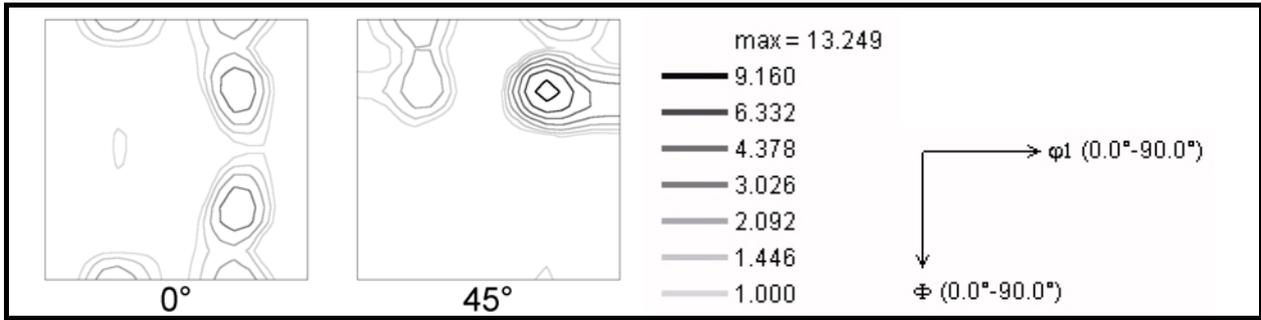
Fig. 3. ODF of intermediate annealed sample measured by EBSD,  $\phi_2$  ( $0^\circ$  and  $45^\circ$ ) sections.
