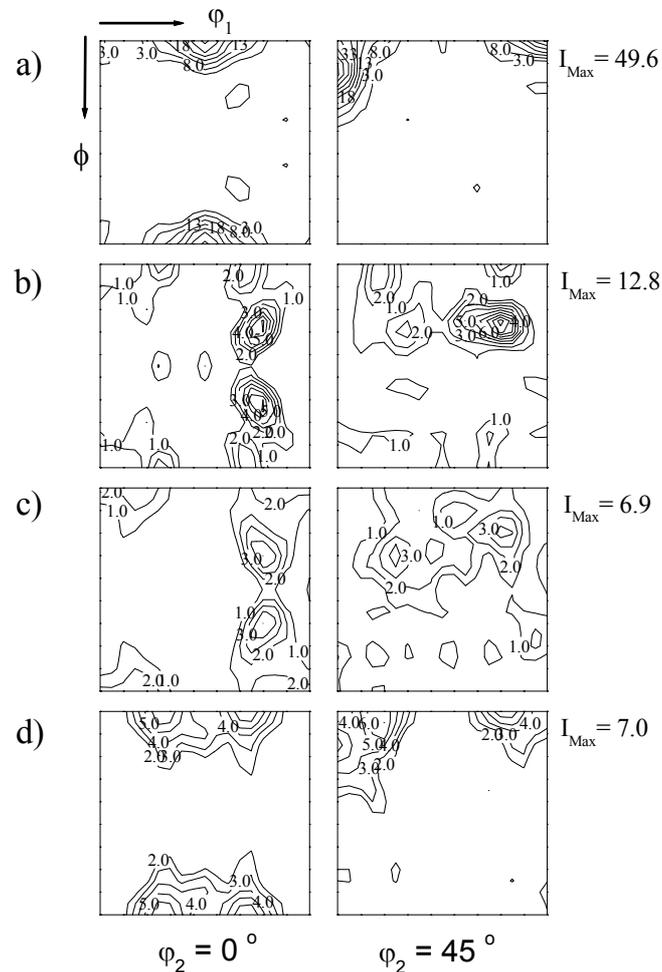
Fig. 2.  $\phi_2$  constants sections ( $\phi_2 = 0^\circ, 5^\circ, 10^\circ, \dots, 90^\circ$ ), of the sample after cold rolling (a), intermediate annealing (b), second cold rolling (c), and final annealing (d)
