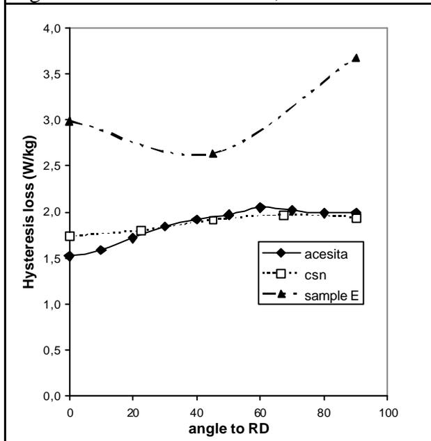
Figure 4. Hysteresis loss at 1.5T, 60Hz
