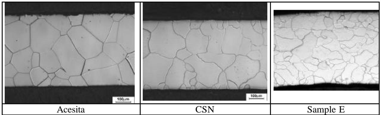
Figure 1. Microstructure of the three samples shows wavy grain boundaries in the annealed semi-process steels and straight grain boundaries in the fully processed steel.
