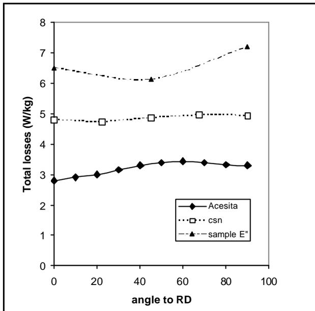
Figure 2. Total losses at 1.5T, 60Hz
