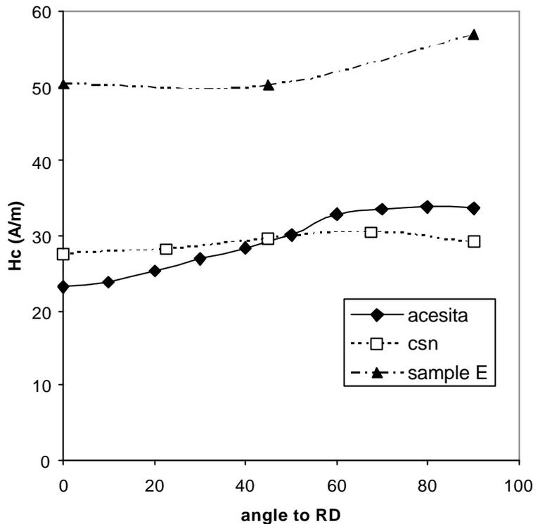
Figure 10. Coercive force from 1.5T, measured at 0.005Hz.
